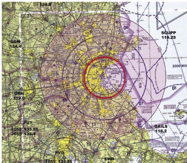
Figure 5-16. A temporary flight restriction (TFR) imposed at Boston's Logan Airport to general aviation and restricting operations at surrounding airports.
