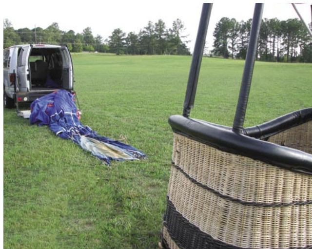
Figure 6-8. Unloading the basket and moving the vehicle forward minimizes equipment carrying.
