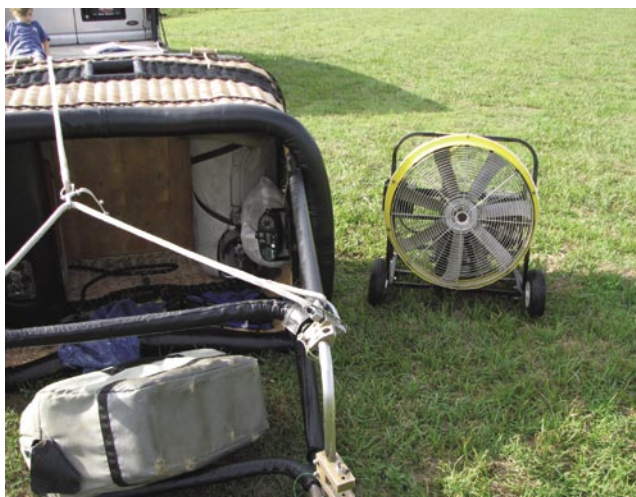
Figure 6-13. Placement of the inflation fan.
