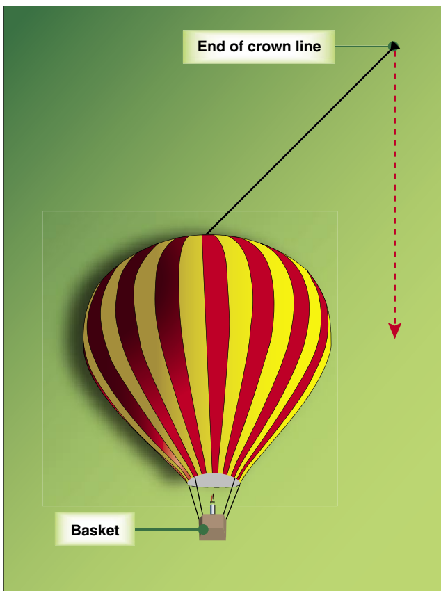
Figure 6-5. Crew can often stabilize a rolling envelope by taking a single crown line 45° off of downwind and walking directly upwind on stand-up.
