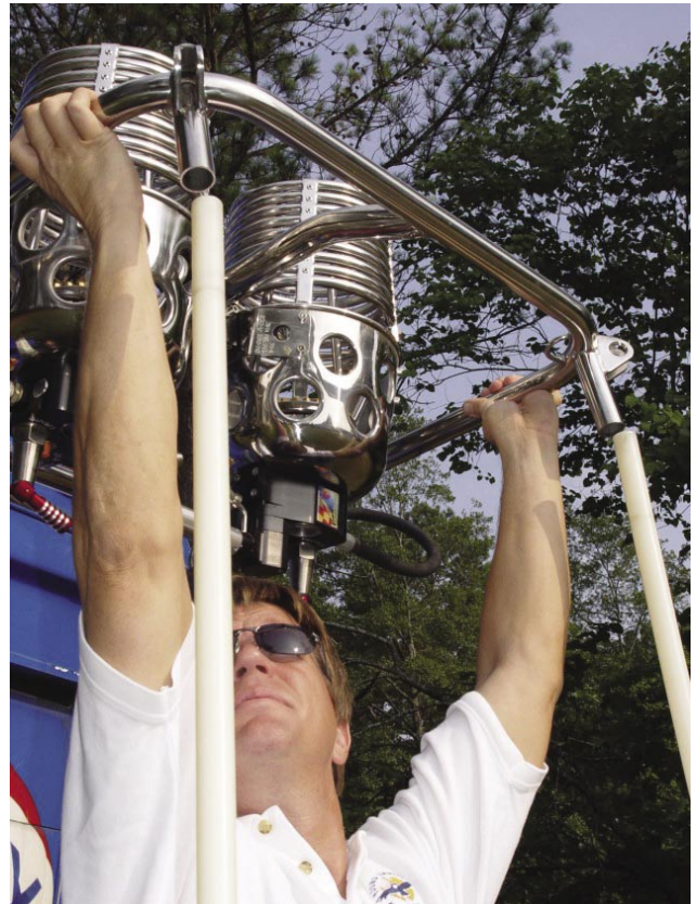
Figure 6-9. Burner installation on a Lindstrand.
